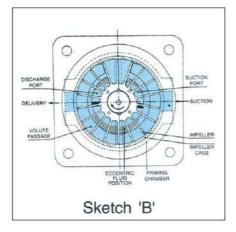
Once past the bridge, however, the liquid between the impeller blades is thrown out into the volute passage which increase in cross-sectional area.
