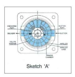
The rotation of the impeller throws the liquid out between the blades towards the periphery by centrifugal force and at the same time imparts velocity to the liquid in the volute passage. The air being lighter remains in the center of the cage. The volute has its maximum cross-sectional area between points at the bottom section of the impeller cage and decrease in area in either direction from this point.
